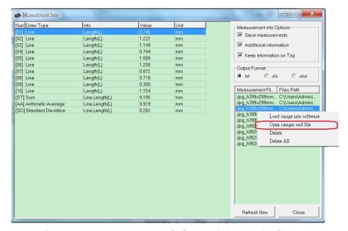
Note: 1) must set Measurement info first and choose the file user want to save, such as txt file or excel file. Note: 2) when click on different output format, it will show the files which saved under this mode. If you have 10 files, but only 3 in txt file, then you can only see 3 files under txt list.
